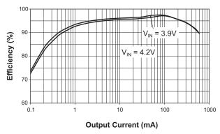
Step-Down Converter DC Regulation ( $V_{OUT} = 3.3V$ ; L =  $10\mu$ H; ENLDO = GND)
