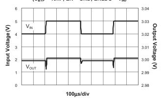
LDO Load Transient Response (C<sub>BYP</sub> = 10nF; EN = GND; ENLDO = V<sub>IN</sub>)
