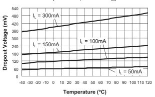
LDO Dropout Characteristics (EN = GND; ENLDO = V<sub>IN</sub>)
