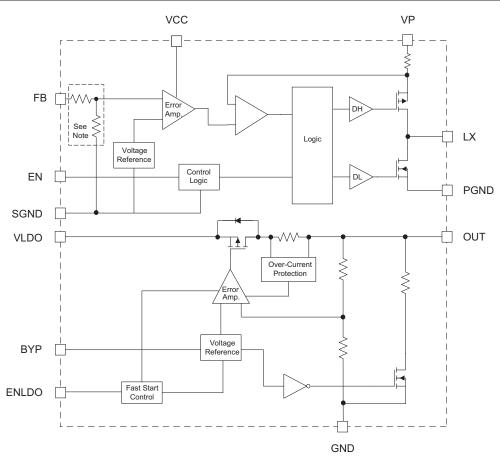
Note: Internal resistor divider included for  $\geq 1.2V$  versions. For low voltage versions, the feedback pin is tied directly to the error amplifier input.
