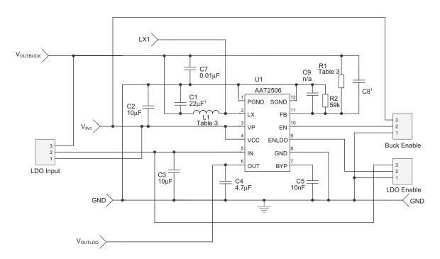
Figure 5: AAT2506 Evaluation Board Schematic.
