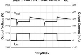
LDO Load Transient Response 300mA (C<sub>BYP</sub> = 10nF; EN = GND; ENLDO = V<sub>IN</sub>)
