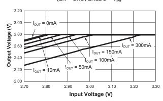
LDO Dropout Voltage vs. Output Current (EN = GND; ENLDO =  $V_{IN}$ )
