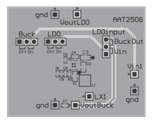
Figure 4: AAT2506 Evaluation Board Bottom Side.
